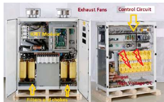
Figure 70: Central inverter internal structure
