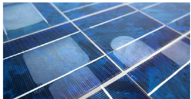
Figure 34: Tiny Hairline Cracks
