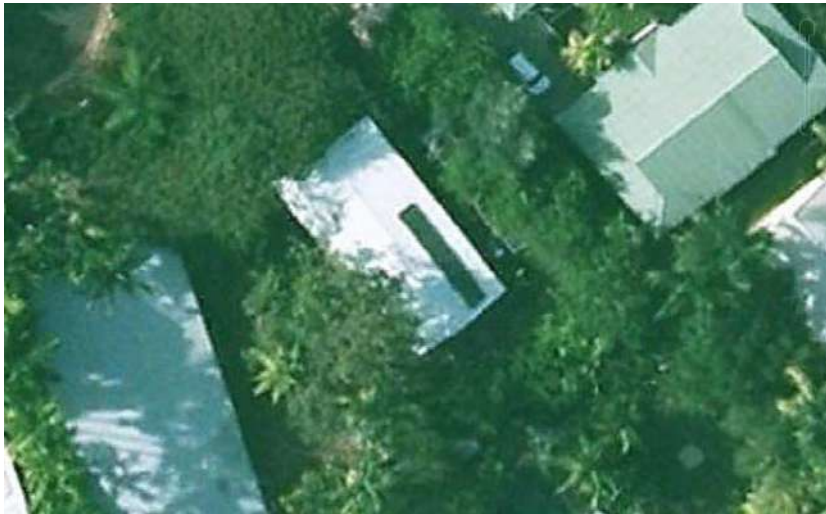
Figure 29: Shows the partial shading on a residential installation
