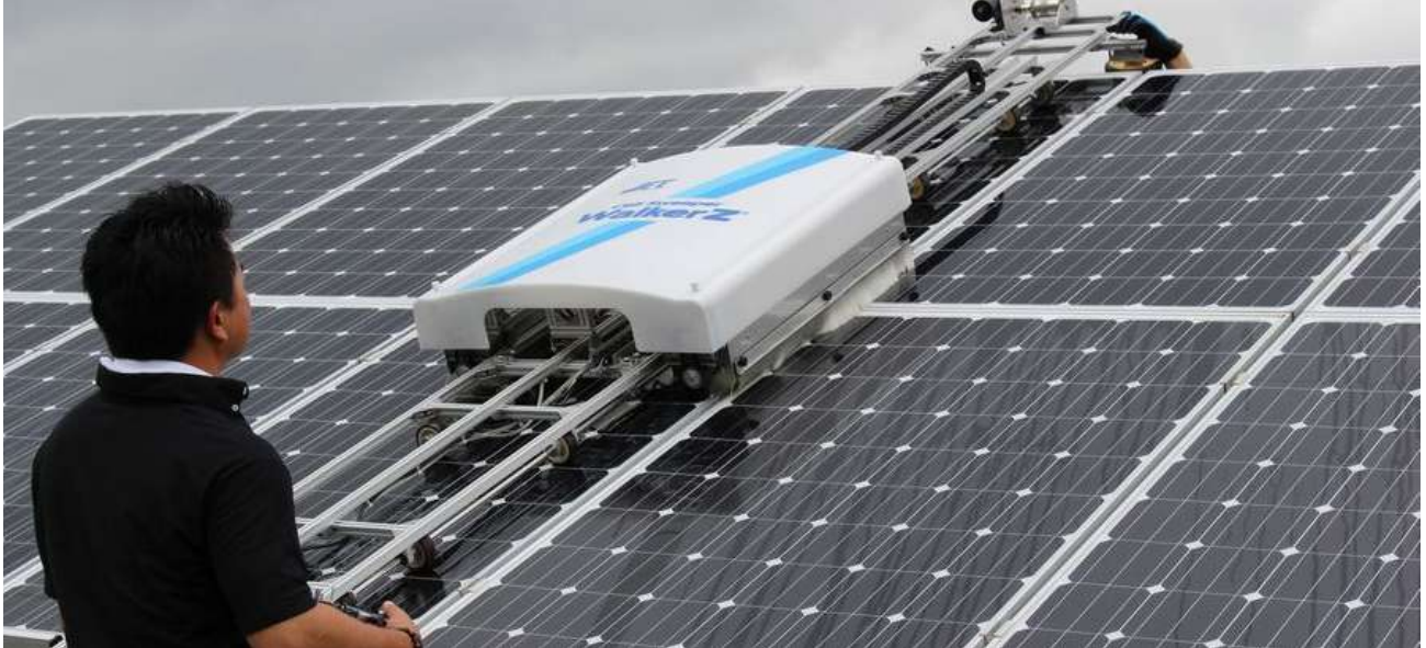
Figure 44: Wet cleaning using Robotic Method
