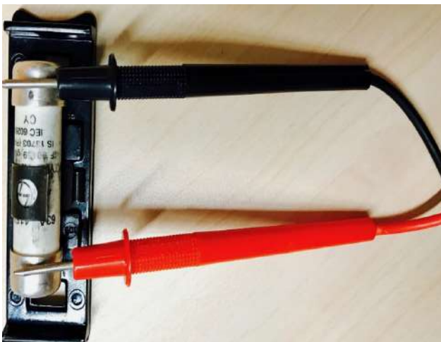
Figure 143: Fuse testing using Multimeter
