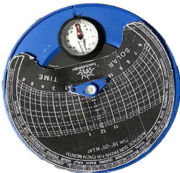
Figure 55: Solar Pathfinder indicating latitude location
