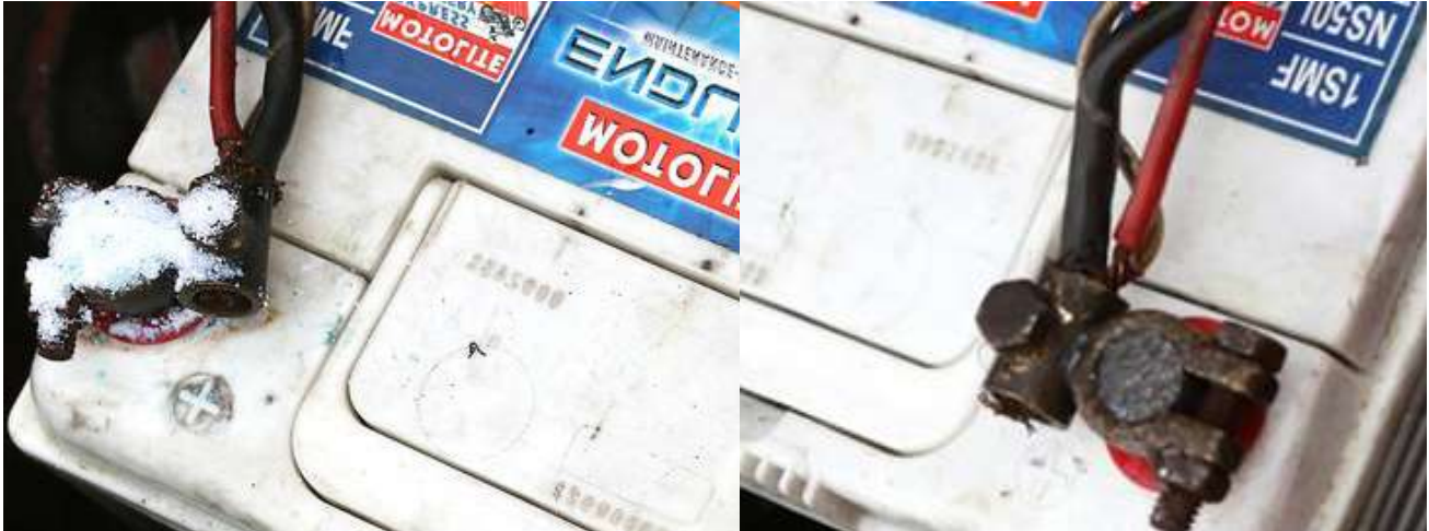
Figure 129: Improper and proper battery terminals
