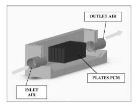
through the stored cooling in the Thermal Energy Storage (TES) system.
